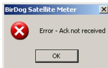
If you get this error message "Error – Ack Not Received". Check that the USB interface connection is correctly made and that the USB cable is undamaged.
